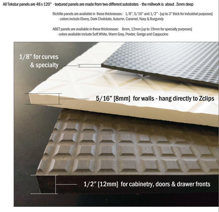
All Tekstur panels have a balancing grid milled on the back face - with the exceptiopn of 1/8" intended for layup with epoxy
