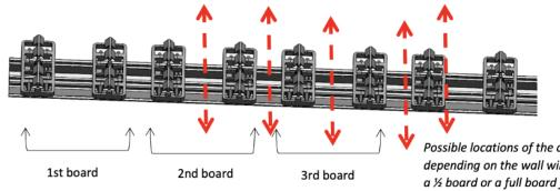
Possible locations of the cuts depending on the wall will finish with a ½ board or a full board face. It is possible to cut right on the edge a clip
