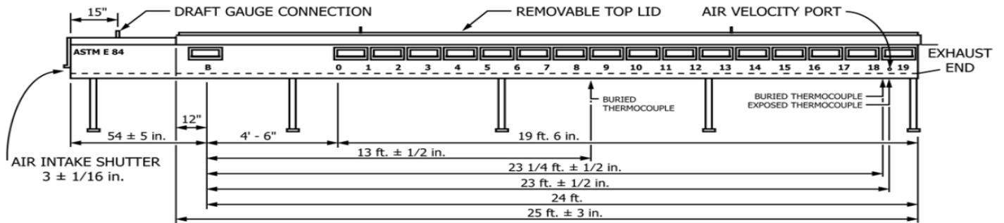
Diagram 1. Test Chamber side view showing critical dimensions.
