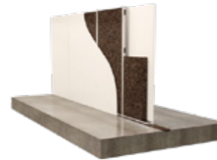
Internal partitions Metal-stud wall and slab discontinuity
