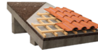
Roofs Pitched roof with roof membrane
