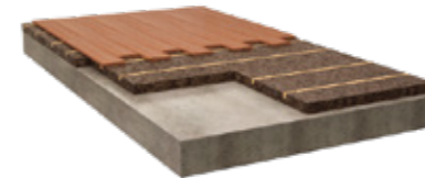
Slab and Floors Lightweight concrete - screed filling
