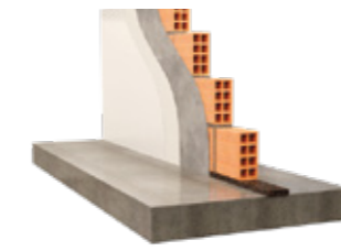
Internal partitions Masonry wall and slab discontinuity
