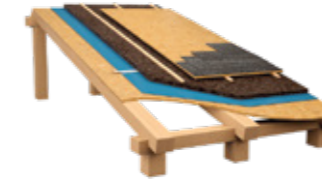
Roofs Pitched roof with above rafter insulation
