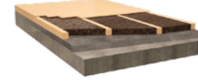
Slab and Floors Unlinking screed filler to the wall
