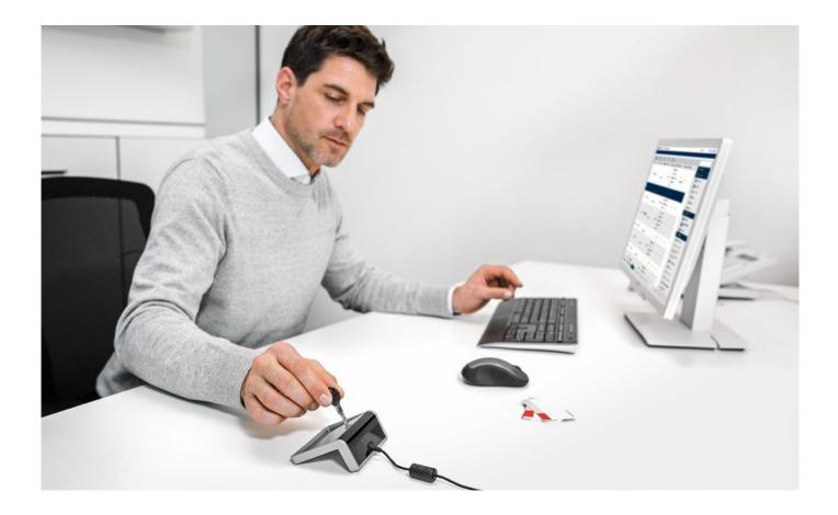
The dormakaba desktop reader 91 08 reads and writes RFID media in the form of cards, smart keys or key fobs that are used for time recording or access control. The desktop reader is connected to a PC via its USB port. The device is automatically detected and installed by Windows.
