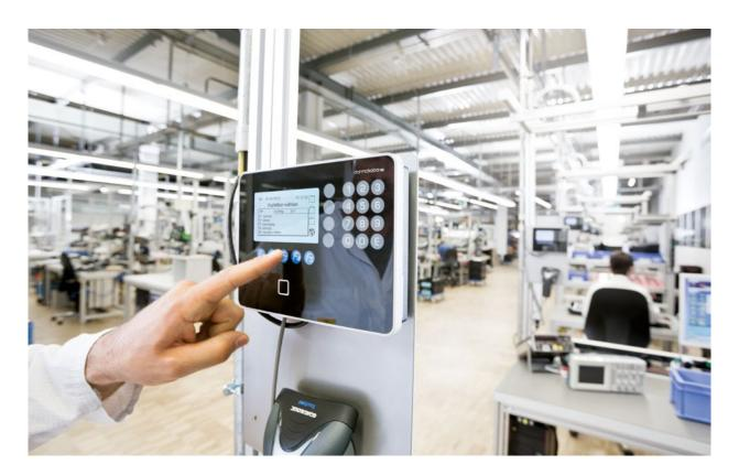
The Terminal B-eco offers a user-friendly solution with identification via RFID card, badge reader or biometric fingerprint for all data collection tasks and the collection of job data using a CCD barcode reader.
