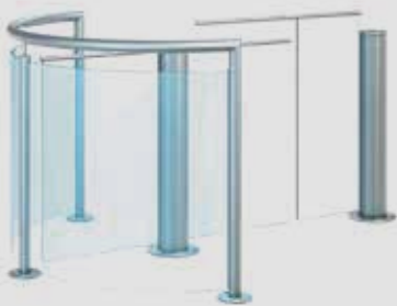
Charon HTS-M01 Turnstile with swing door, high glass elements and stainless steel push bars. Turnstile with 180° turn cycle for person separation and transport opening as soon as the turnstile and swing door are opened together at 90°.
