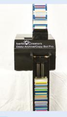
**D2** The old disk duplicator came with two attachable hoppers, each capable of holding 50 floppies. The disks are stacked in the input hopper and the Raspberry Pi controls when a disk is inserted into the duplicator's built-in disk drive.
