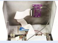
**D3** The Greaseweazle device extracts the raw flux transitions from a drive to capture the disk format and sends the data for storage on the Raspberry Pi. The disk is ejected and a spring-loaded mechanism in the output hopper limits its fall.
