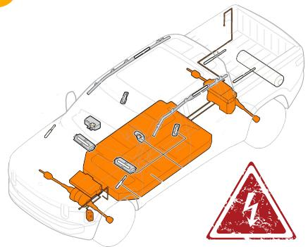
Avoid airbags, HV lines, hydraulic lines and compressed air tanks. **You could be injured, electrocuted, or die if you cut, pierce, or damage the highlighted areas.**
