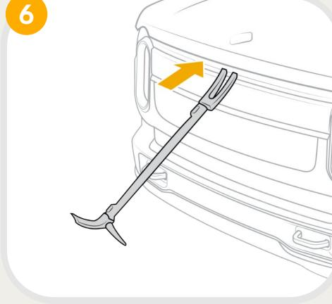
To **gain access to the first responder loop**, the hood can be forced open using a Halligan bar and a hydraulic spreader at the latch in the middle of the hood.
