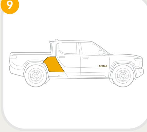
The gear tunnel on an **R1T** can be forced open with a Halligan bar and spreader. The door to the tunnel is hinged at the bottom with a latch at the top.
