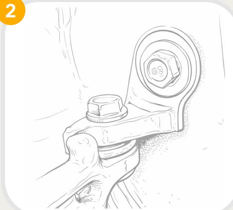
To remove the doors, expose the hinges at the front of the door. Use a hydraulic cutter for the hinges and a spreader to force the door open.
