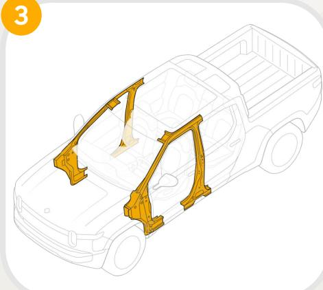
Use a hydraulic cutter or reciprocating saw with a diamond blade to cut steel around doors. Cut higher than typical - the seat belt slider and anchor bolt mechanism sits high.
