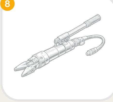
Dash lifts can be done using a spreader or hydraulic ram. Support the tool in the door sill area. Using the tool inside of the sills can puncture the vehicle battery.
