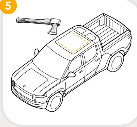
If the vehicle has a glass roof, it can be cut away with an ax or a sawzall.
