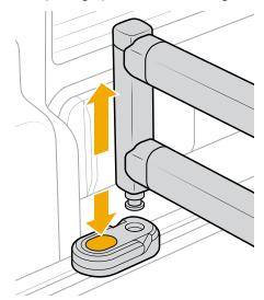
2. Push the cargo divider legs inward to collapse the divider.
