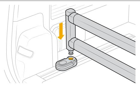
7. Move the cargo tie-downs along the rails to reposition the cargo divider. Lift the hook on each cargo tie-down, and then press down on the black button to move it forward or backward.
