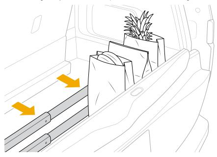
10. Gently push and pull on the cargo divider to confirm that it is securely locked in place.
