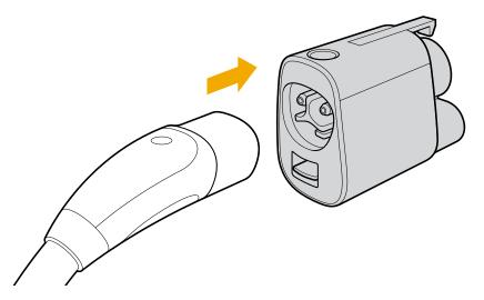
2. Align the adapter plug with the vehicle's charge port, and fully insert the plug into the port. The vehicle starts to charge automatically.
