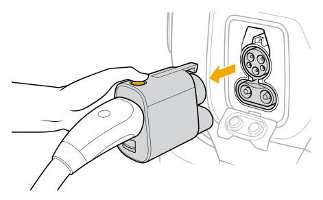
4. Press down on the tab below the NACS adapter port (1) and pull the charge plug out of the adapter (2).
