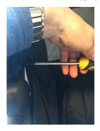
Take a small flat screw driver and gently move under the plastic clip releasing the canopy.
