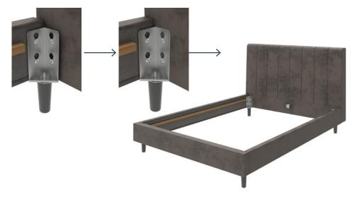
Place the centre rail into headboard and foot end centre brackets. Tighten up the corner brackets from step 8.
