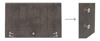
Carefully position headboard screws over the corner brackets and tighten the screws.
