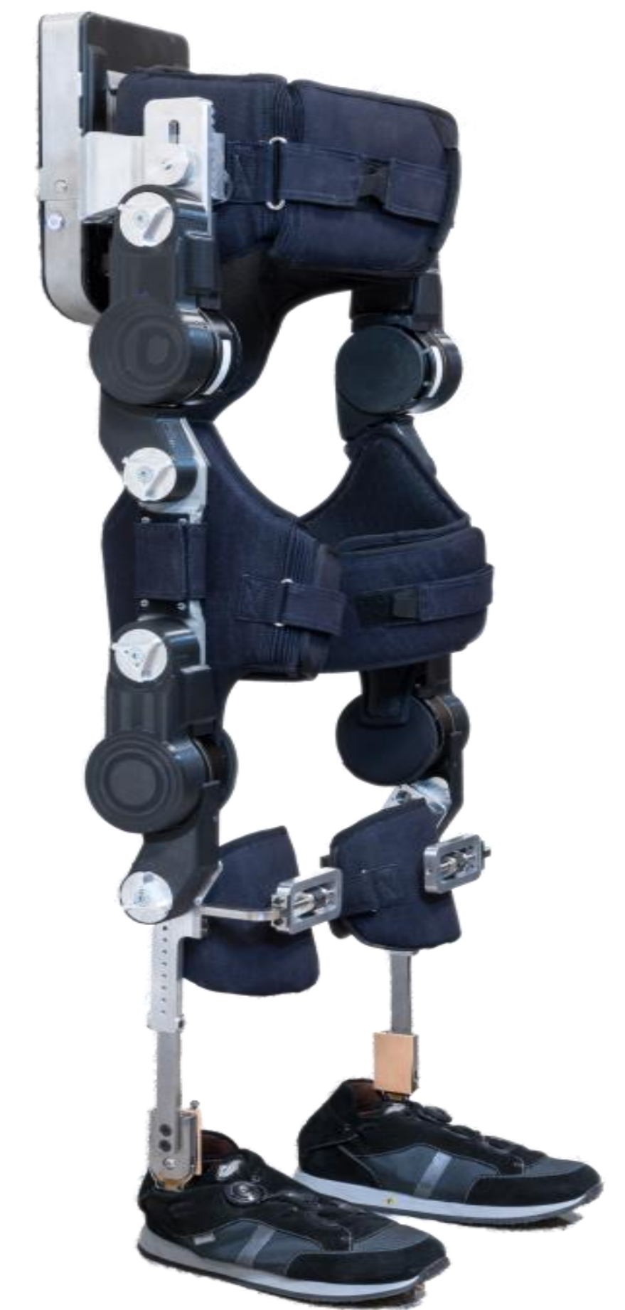
Fig. 1 The TWIN exoskeleton developed at the IIT-INAIL Rehab Technologies Lab.
