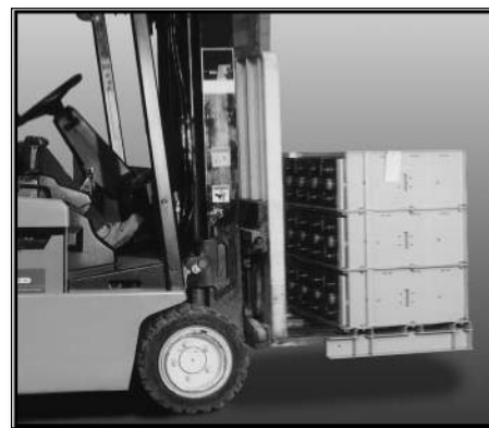
Figure 6-1 Installation Using Forklift
