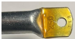
Figure 4.6.3B – Lug with proper no-OX application
