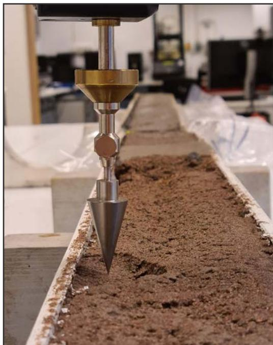
Figure M6. Fall Cone setup, shown before the cone is released into the sediment.
