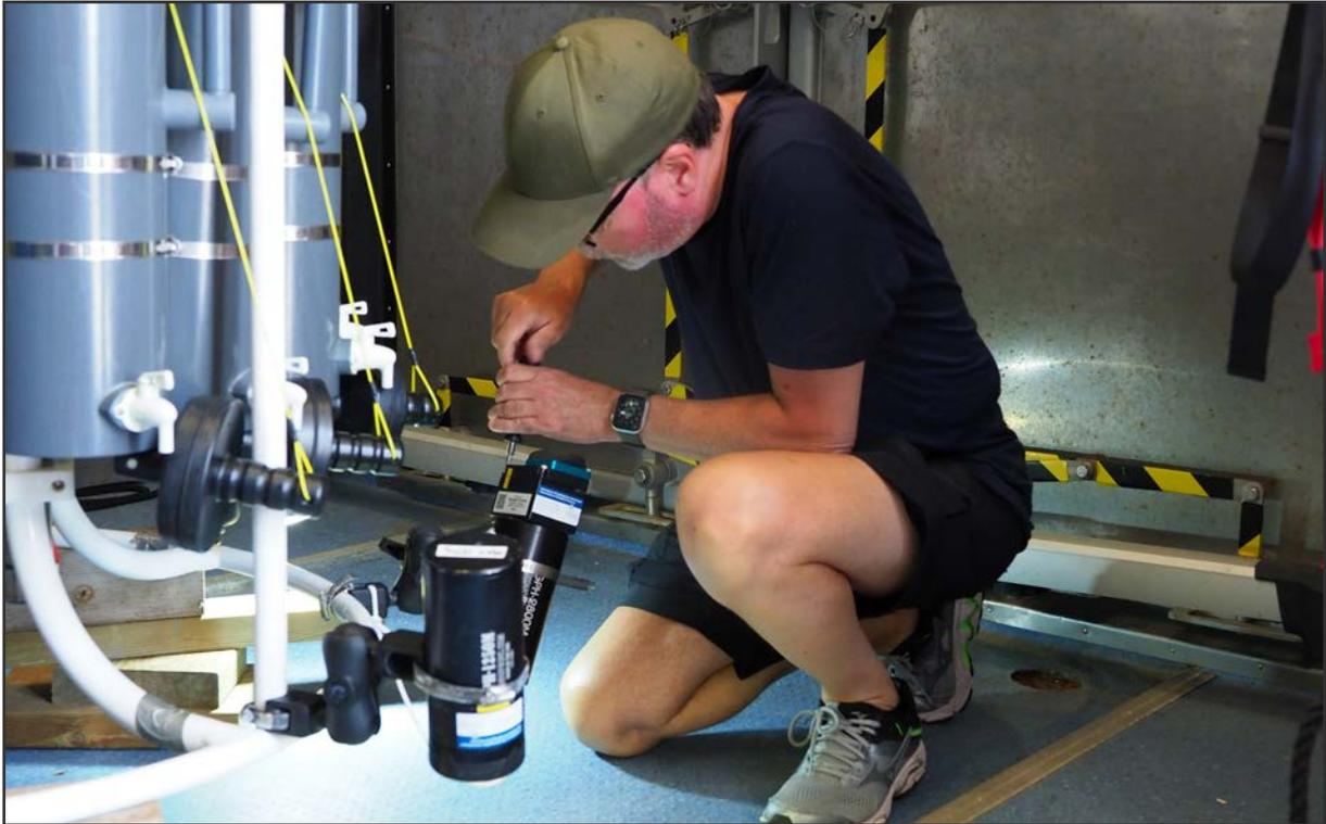
Photo M4. GoPro Hero 7+ camera and light placed in water proof housings and mounted on the frame of the CTD carousel. Bottom inspections were carried out either along with CTD-casts or separately by lowering the carousel to the seafloor. Photo: Martin Jakobsson
