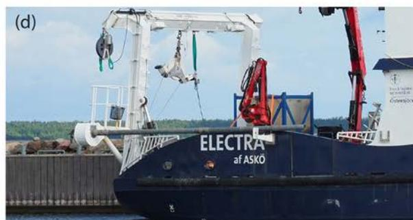
Photo M2. The coring system on RV Electra. (a) The corer has a launching system on the starboard side. A portable refrigerator for core storage is placed on the aft deck. (b) Core head loaded with 473 kg led weights. (c) Coring winch (InterOcean model 10031-20HLW hydraulic) equipped with 600 m of 11.43 mm diameter cable (Rochester A302799). (d) Corer in handling system. Photos: Martin Jakobsson (a and c are reused from previous cruise reports). Photos: Martin Jakobsson
