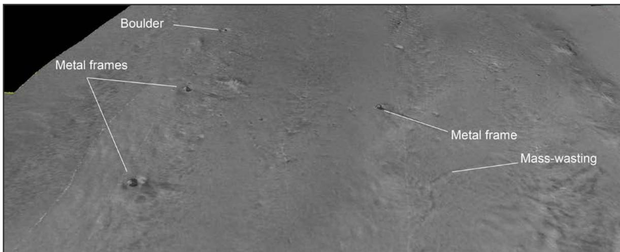
Figure SBI18. 3D-view of backscatter imagery draped on top the multibeam bathymetry in the area where the metal frames are located north of MS Estonia.
