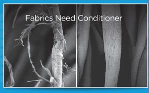
Unconditioned Fibres **Conditioned Fibres**
