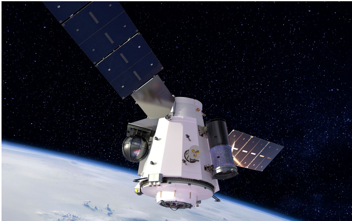
A proposed Unmanned Orbital Outpost leveraging a repurposed Dream Chaser 'Shooting Star' Cargo Module. Smart reutilization of space hardware enables experimentation and logistics while reducing costs and orbital debris. (Source: Sierra Nevada Corp)
