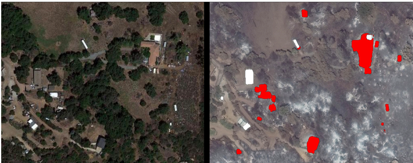
xView2 satellite imagery assessment of a location (right) identifies damaged structures after California's 2020 Valley Fire.
