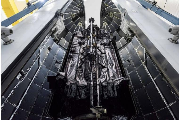
Figure 53: GPS III SV04 is encapsulated within a SpaceX payload fairing on Sept. 21 in preparation for its launch on 29 Sep 2021 from Cape Canaveral Air Force Station, Florida (Credit: Space Launch Delta 45)
