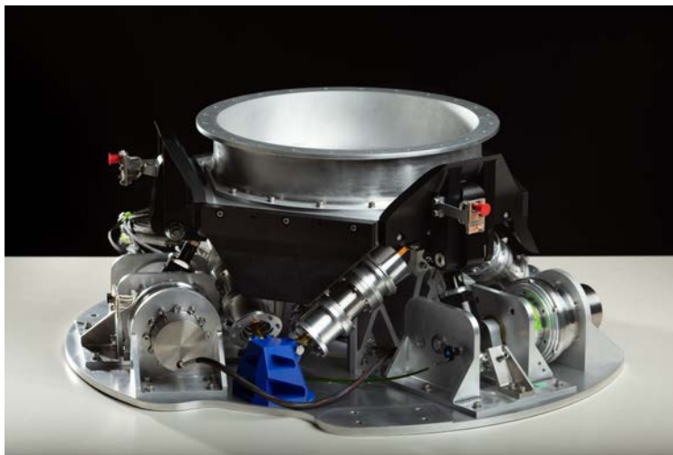
Figure 39: The Augmentation System Port Interface (ASPIN) can dock to existing satellites and add new capabilities to a spacecraft that is already in orbit (Credit: Lockheed Martin).
