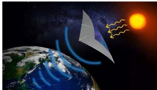
Figure 8: AFRL's Space Solar Power Incremental Demonstrations and Research Project (SSPIDR) is a collection of flight experiments designed to mature critical technologies needed to build an operational solar power beaming system in space transforming energy production & distribution on Earth (AFRL).
