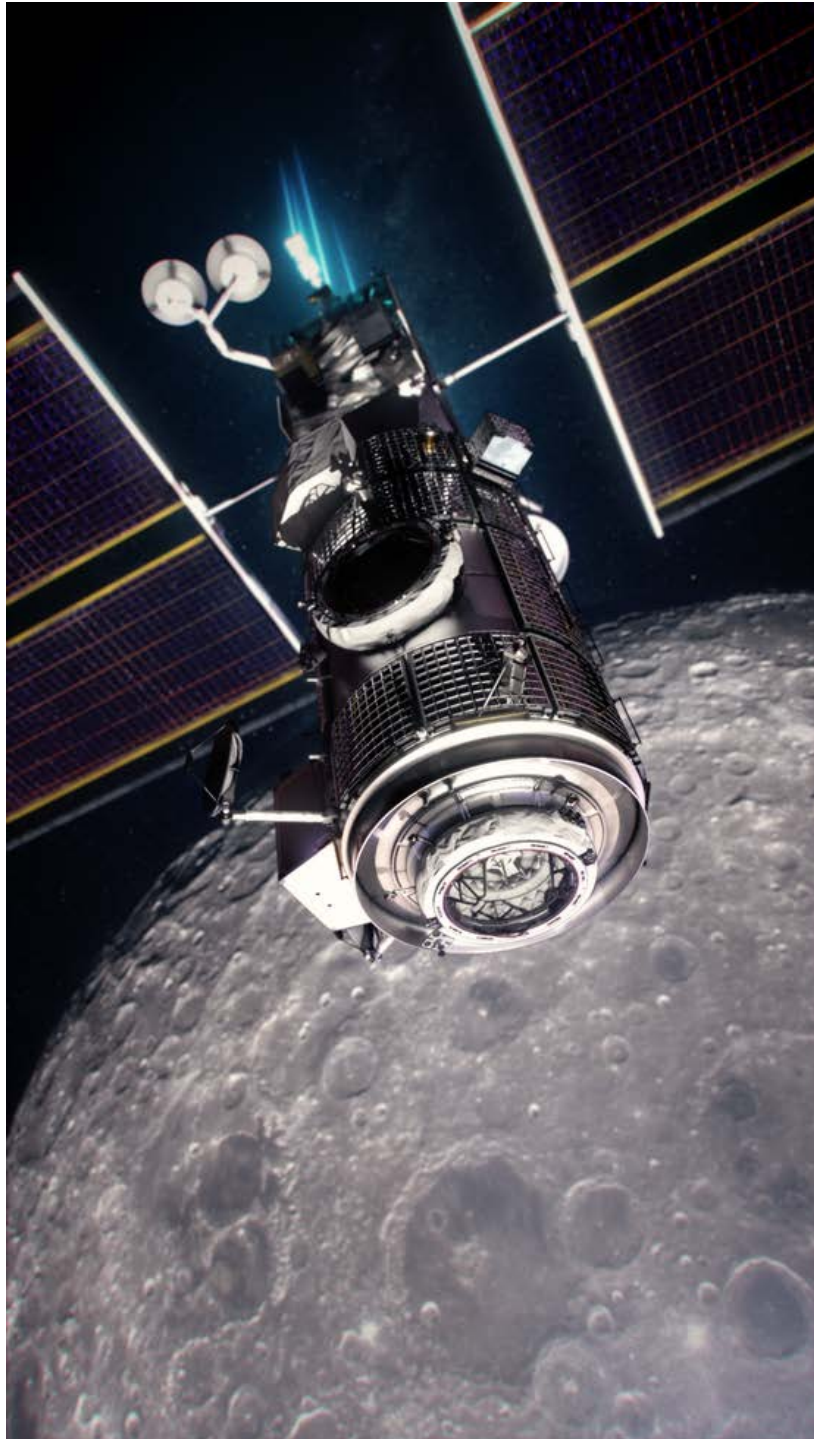
Figure 28: Illustration showing a close-up of the Habitation and Logistics Outpost (HALO), one of the elements of the Artemis Gateway launching no earlier than May 2024 (Credit: NASA).
