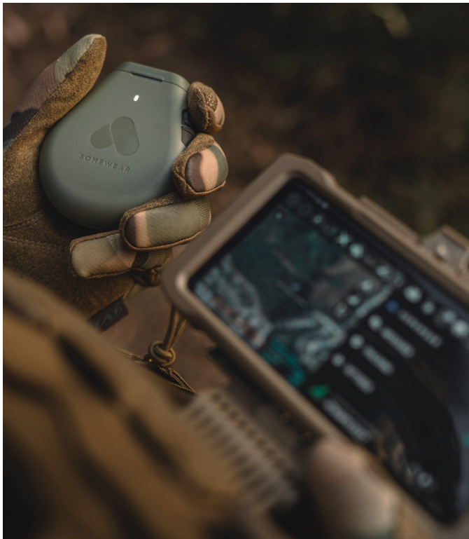
Somewear Lab's satellite communicator paired to a wireless device with Somewear's ATAK plugin. (Somewear Labs, Inc.)
