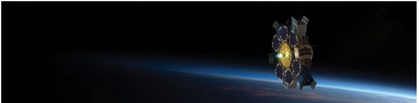
Artist rendering of Apollo Fusion's Hall Effect Thruster integrated on a SpaceFlight Inc. Sherpa-LTE bus (Apollo Fusion)
