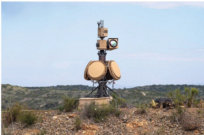
Anduril's Long Range Sentry Tower System for UAS Detection, Tracking, and Identification (Anduril)
