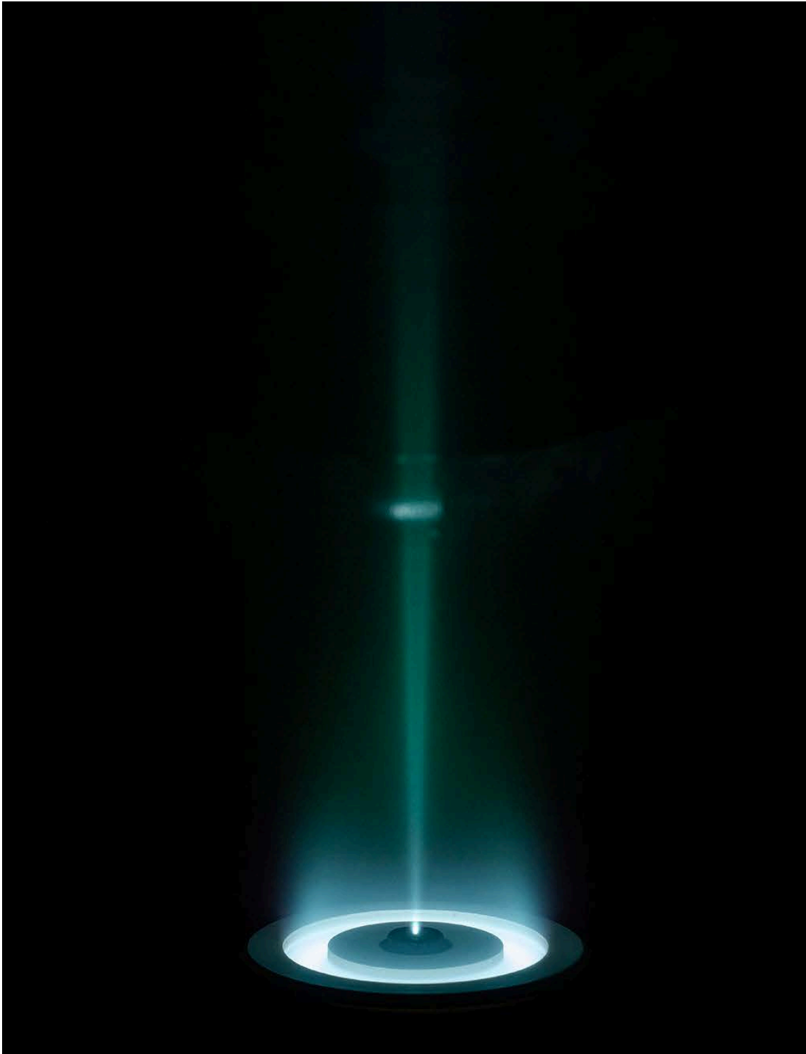
Figure 18. Hall Effect thrusters are the first step toward achieving dynamic space operations (Credit: Astra)
