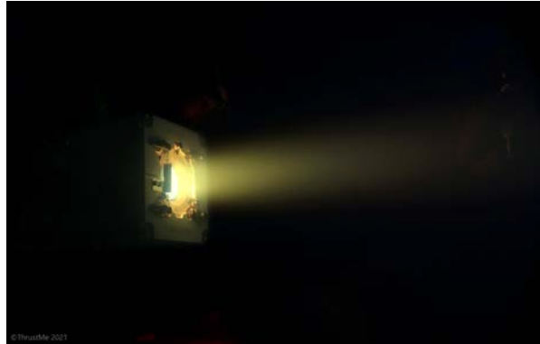
Figure 20. The Norwegian Space Agency's NorSat-TD satellite is fitted with a ThrustMe NPT30-I2 iodine fueled electric propulsion system. (Credit: Thrustme 129 )
