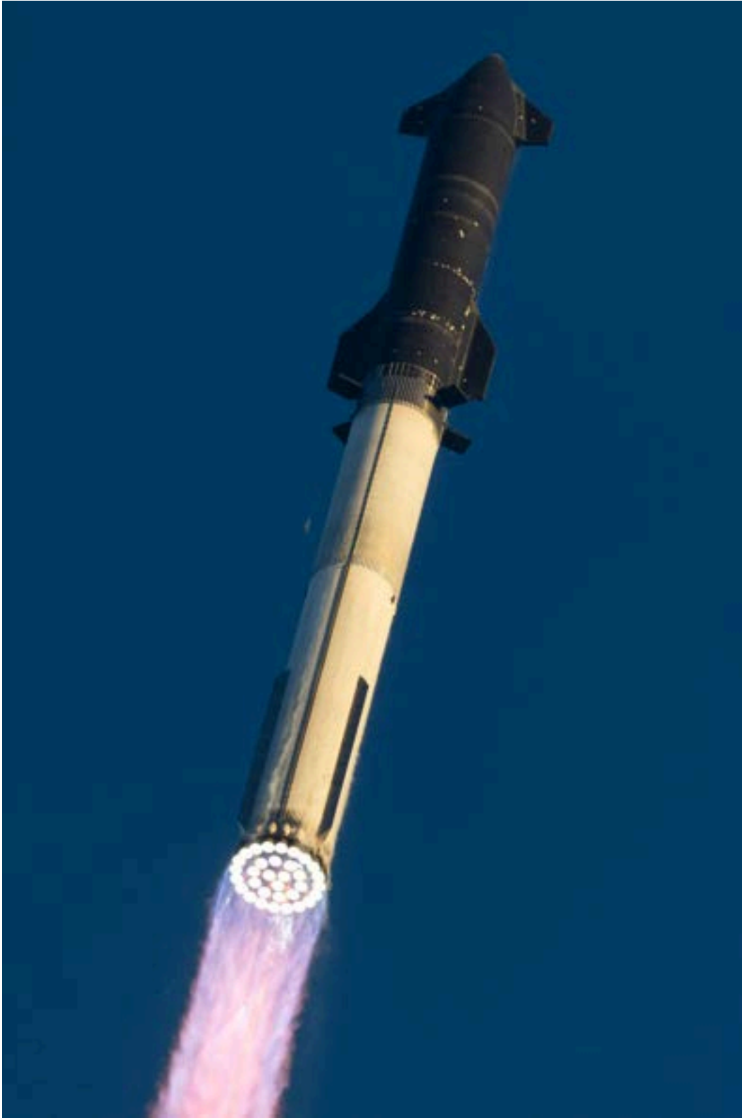
Figure 24. Starship launches off the pad under the power of all 33 Raptor engines on the Super Heavy Booster during Test Flight 2 on 18 Nov 2023. (Credit: SpaceX)
