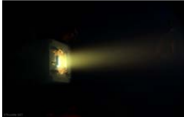
Figure 20. The Norwegian Space Agency's NorSat-TD satellite is fitted with a ThrustMe NPT30-I2 iodine fueled electric propulsion system. (Credit: Thrustme 128 )
