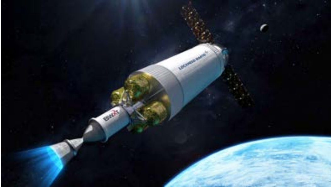
Figure 22. Illustration of the DRACO spacecraft being developed by Lockheed Martin for DARPA that will demonstrate thermal nuclear engine technology. (Credit: Lockheed Martin)
