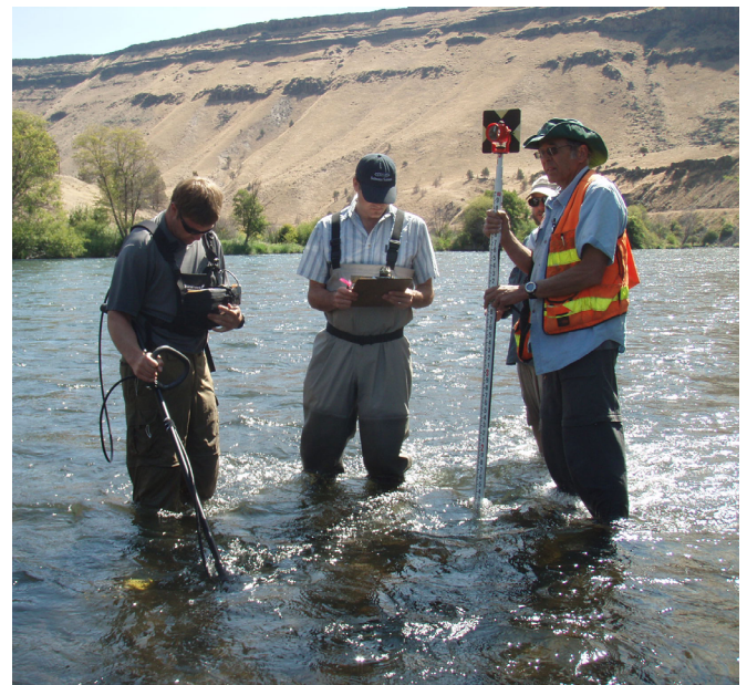
In Phase 1 of the gravel study, tagged tracer rocks were surveyed, providing information on river flows and use by spawning salmon.
