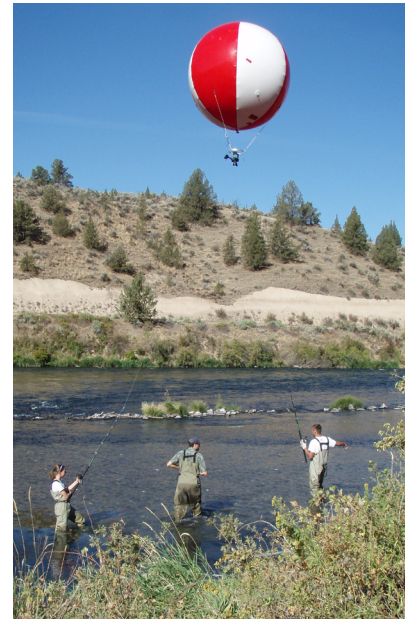
A digital camera suspended from a weather balloon was used to take high-resolution images of our gravel augmentation study sites.
