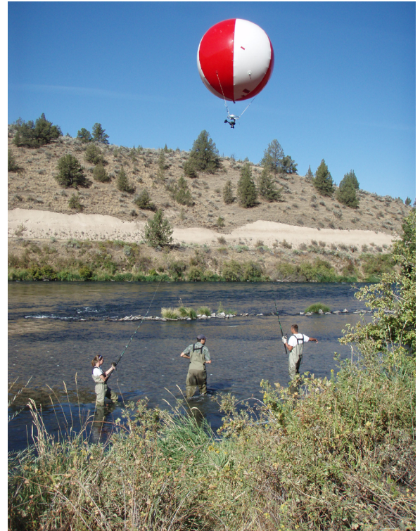
A digital camera suspended from a weather balloon was used to take high-resolution images of our gravel augmentation study sites.
