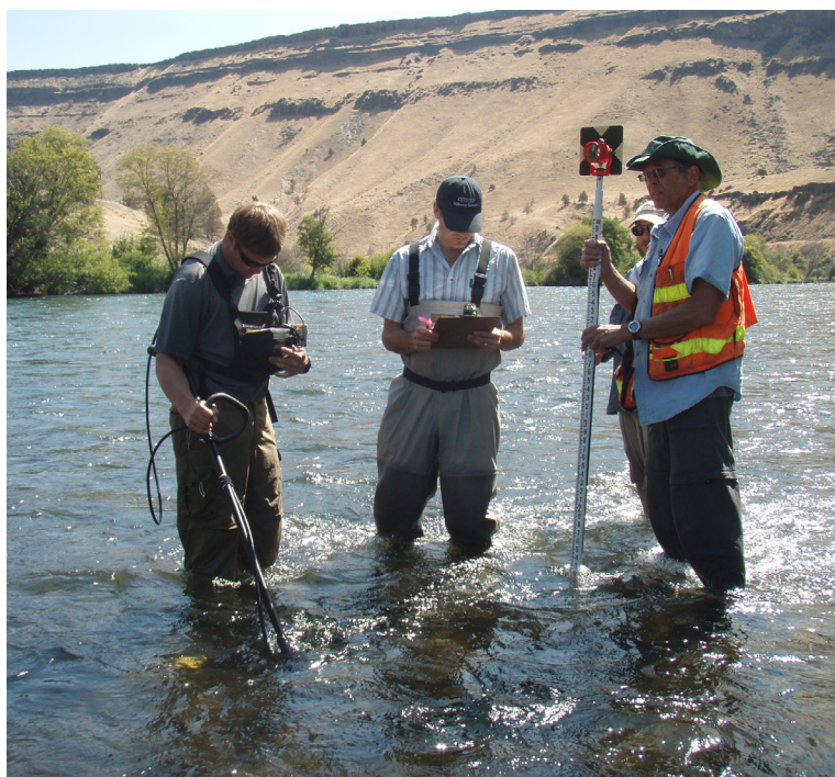
In Phase 1 of the gravel study, tagged tracer rocks were surveyed, providing information on river flows and use by spawning salmon.
