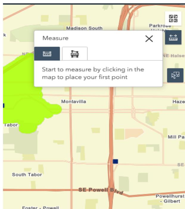
A. Measure a distance: click the **distance** button ->click two or more points on the map to draw a line. When you are finished drawing, double-click to complete the line. The result of your distance measurement appears at the bottom of the Measurement tool. To change the distance unit, choose a new unit of measurement from the drop-down menu. To measure another distance, click on the map and draw a new line.
