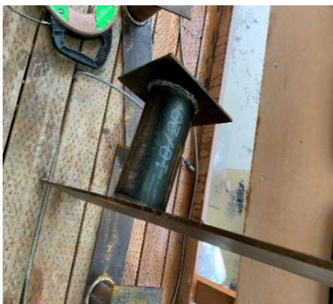
Figures 10 and 11. 8-inch × 8-inch × ¼-inch Base Plate, 4-inch Diameter × ¼-inch-Thick Tubing, and 28-inch × 8-inch × ¼-inch Plate
