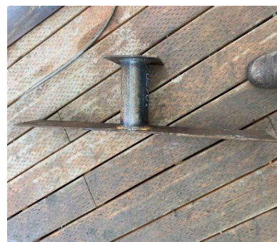
Figures 10 and 11. 8-inch × 8-inch × ¼-inch Base Plate, 4-inch Diameter × ¼-inch-Thick Tubing, and 28-inch × 8-inch × ¼-inch Plate
