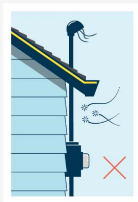
Bent or frayed wires. DO NOT TOUCH.
