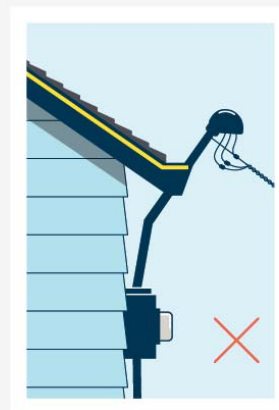
Bent or broken weatherhead.
