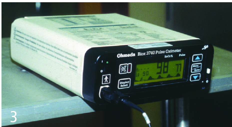
Pulse oximeter displaying pulse waveform, rate, and oxygen saturation ( SpO_2 )
