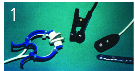
Probe types: Transmittance (left 2 probes) and reflectance (right 2 probes)
