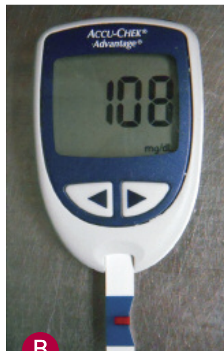
Adding blood to a test strip of a blood glucose monitor (Accu-Chek Advantage, roche.com) (A) and the resulting blood glucose level in mg/dL (B).
