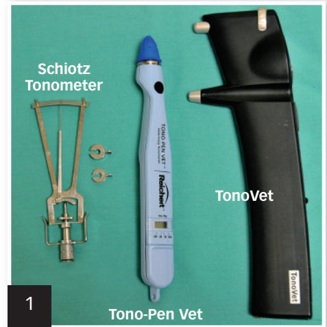
Three tonometers commonly used in veterinary medicine are the Schiottz indentation tonometer, the Tono-Pen Vet applanation tonometer, and the TonoVet rebound tonometer.
