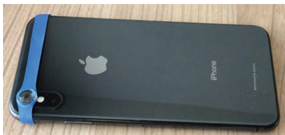
▲ FIGURE 4 Mounted appearance of a macro lens (Easy-Macro) to an iPhone XS Max. The flash component of many smartphones is aligned horizontally, rather than vertically, as shown here; this may obscure the flash and require the examiner to provide independent illumination (eg, penlight) to the eye.
