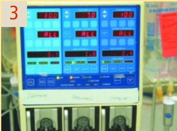
3 The Trilogy Multichannel Infusion pump ($4000, Medex, Inc., Carlsbad, CA) can simultaneously deliver three fluid types at three different rates.
