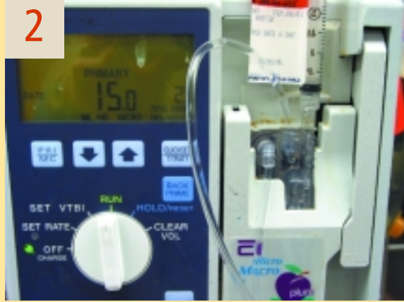
2 The Abbott Plum XLD IV pump ($2389; Abbott Laboratories, Abbott Park, IL) contains a primary and secondary function so that a secondary infusion can be programmed for administration. This pump cannot deliver both infusions simultaneously.
