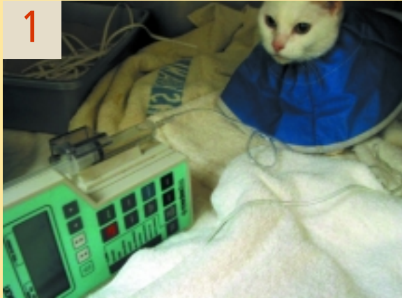
1 The Medfusion 2010 Syringe pump ($2200; Medex, Inc., Carlsbad, CA) can accurately deliver drugs in syringes ranging in size from 3 to 60 ml.
