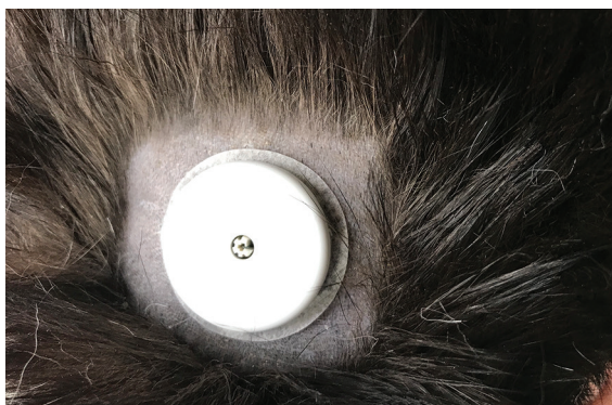
▲ FIGURE 1 A sensor unit from a flash device adhered to the skin of a diabetic cat. A manufacturer-provided device easily applies the small sensor unit (35-mm diameter × 5-mm height) to the shaved area. The sensor uses a flexible filament in contact with the interstitial fluid to measure BG every 60 seconds and data storage capacity to record BG data. Wireless technology transfers BG data stored in the sensor unit to a handheld reader unit.
