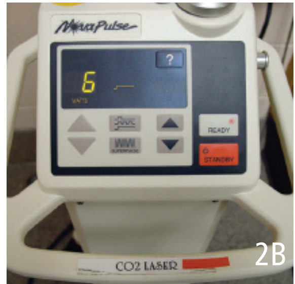
Complete CO 2 laser with handpiece and ceramic tip (h), waveguide (w), and base unit (b) (A); base unit set to 6 W power for continuous laser output (B)
