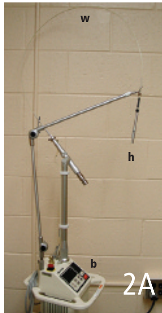
Complete CO 2 laser with handpiece and ceramic tip (h), waveguide (w), and base unit (b) (A); base unit set to 6 W power for continuous laser output (B)
