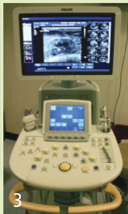
Ultrasound unit with a flat-screen display, 4 transducers (2 linear array, 1 convex, and 1 microconvex), a touch screen, and a relatively simple ergonomic design. A keyboard is located beneath the interface to allow for additional image labeling.
