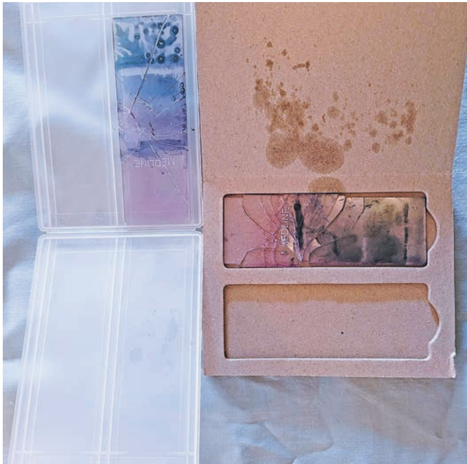
▲ FIGURE 5 Slides broken during shipment due to inadequate protective packaging
