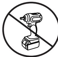
**WARNING:** Never use an impact gun for wall screws. Minimum torque force of 60 inch pounds to maximum of 85 inch pounds.
