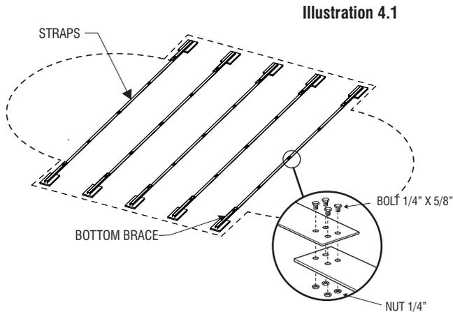
**3) Refer to Illustration 4.2.:** Attach the assembled tension straps to bottom braces on both sides, using four (4) bolts and nuts (BB) 1/4" #20 X 5/8" (6,35 mm X 15,88 mm), taking care of placing the bolt head on top.
