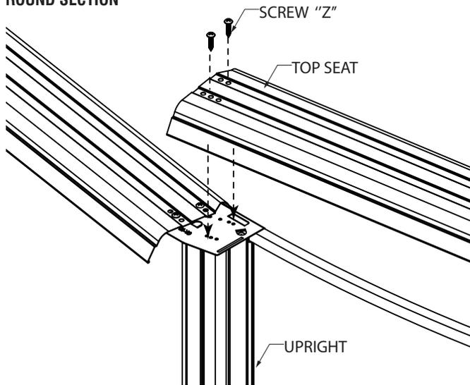
Secure the top seat in place using four (4) screws "Z".
