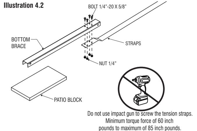
Do not use impact gun to screw the tension straps.
