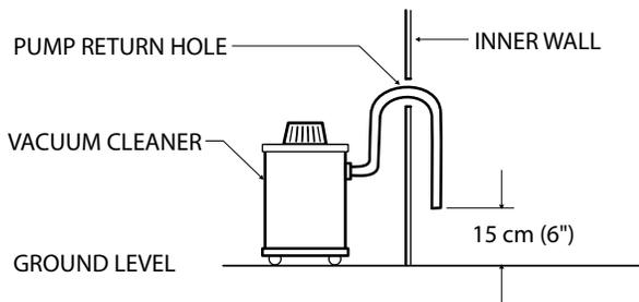
Maintain the hose in place with adhesive tape. Don't forget to block the skimmer hole with adhesive tape to prevent air from leaking in.
