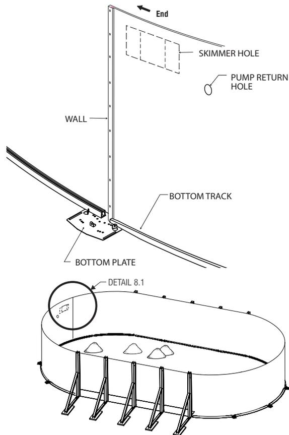
Join both ends of the wall by orienting folds outward to hide the exclamation icon. (Illustration 8.1)
