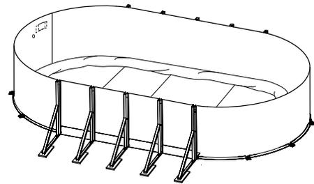
Carefully unfold the liner, bringing the bottom-sidewall seam close to the wall base. Make sure that the side with the protruding seams faces downward or that the patterned side faces upward.
