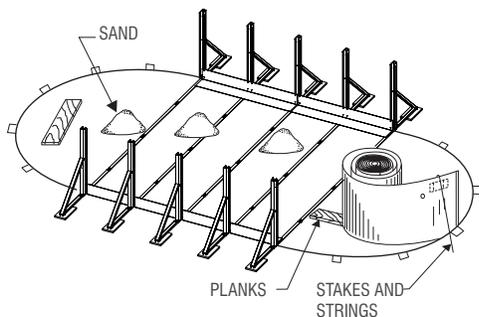
Begin inserting the wall into the bottom tracks in the middle of a bottom plate. At first, the wall is kept in place with one or two stakes and strings (or extra persons). One person uncoils the wall on a beam or a plank, while a second person inserts it in the bottom tracks. Do not uncoil more than 3 m (10') of wall before you install a support bar or stake and string to reinforce the structure.
