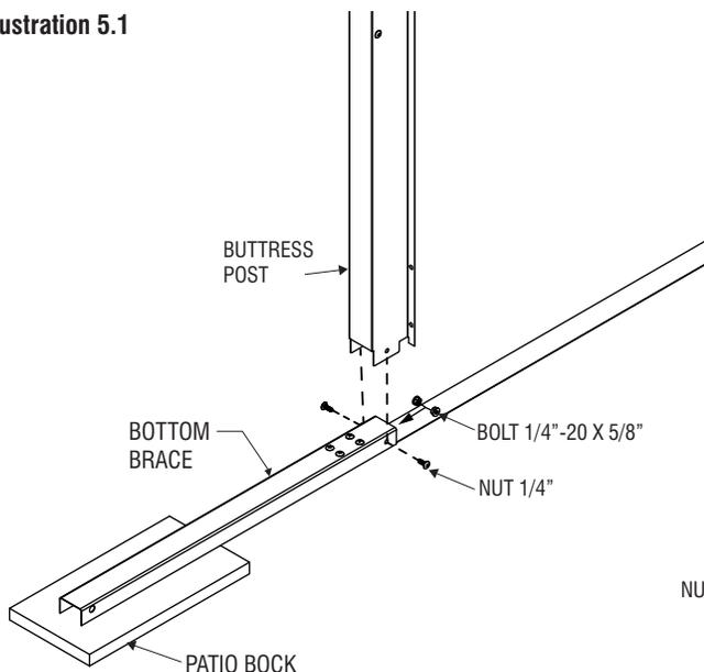
Next, assemble the other side of the angle brace to the buttress post with two (2) bolts and nuts (BB) 1/4" #20 X 5/8" (6,35 mm X 15,88 mm).
