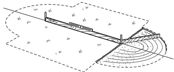
In order to ensure proper water drainage around the pool, a 2-degree slope needs to be erected around the perimeter of the pool. THE MANUFACTURER WILL NOT BE HELD RESPONSIBLE FOR ANY LIABILITY SHOULD THIS STEP BE OMITTED.
