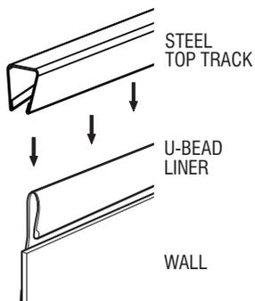
Start the vacuum cleaner to allow the liner to adhere to the wall and check for excess tension at the bottom or for wrinkles. Adjust the liner by removing wrinkles if needed, lift or lower it in order to ensure a perfect fit.
