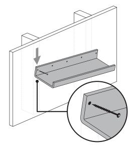
Level the picture ledge and set second screw in opposite end screw hole with your drill. If the screw holes miss an available stud see Rad Tip #1 below. If you've already installed blocking behind the length of the backbar, skip to Step 5.
