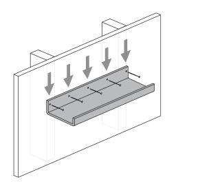
Make final inspection of the picture ledge. Check for picture ledge sag, confirm the picture ledge is correctly secured to wall. If your picture ledge is sagging, refer to Rad Tip #1 and #2.
