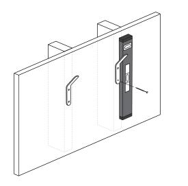
For installation into drywall only, Position hook in desired location. Level the hook, and mark both screw hole locations with a pencil or screw tip.
