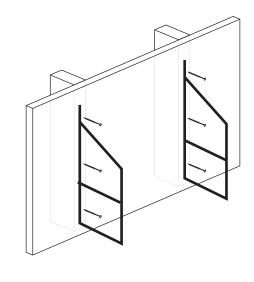
Lay the top shelf on your bracket and position as desired. See Rad Tip #4 below. Hold the bracket perpendicular to your wall by using a square. Hold the shelf steady and install shelf screws into the shelf.
