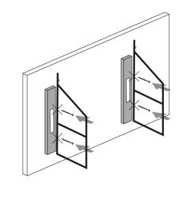
Remove the brackets from your wall. Predrill all marked screw locations with a 1/4" bit and install sheet rock wall anchors in each screw hole location. Take a swig of your brew.
