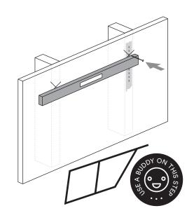
Install all the top screw locations. Vertically level each bracket. Punch a hole in all remaining screw locations with screw tip. If your brackets are on studs or blocking, skip to step 6. If not, proceed to step 5.
