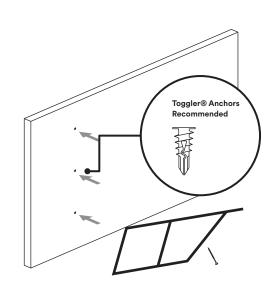
Position the brackets, install all wall 6 screws. Confirm the brackets are secure to wall. Note: Brackets may wiggle left to right at this point. Chill, installing the shelves will resolve this!
