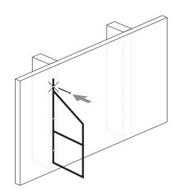
Measure the bracket spacing from screw hole and righteously apply painters tape to general mounting area of second bracket. Measure again and draw a short vertical line on the tape. See Rad Tip #2 below.
