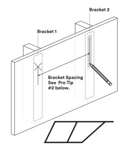
Place a level on first screw hole. Find the intersection at level and vertical line. If you do not have a long enough level, see Rad Tip #3 below. Use a wall screw to punch a hole into wall behind painters tape. Remove the tape.
