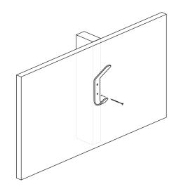
Position hook on the wall in desired location. Mark one screw hole with pencil or screw tip. Predrill this hole with ¼" drill bit to avoid breaking wall anchors.
