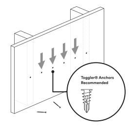
Replace bracket, drill screw into each screw hole and confirm bracket is correctly secured to the wall.\* See Rad Tip #3 below.
