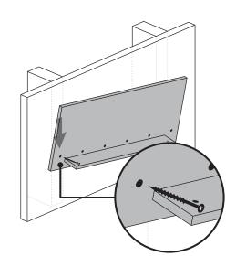
Level bracket and set second screw in opposite end screw hole with your drill. If bracket screw holes miss an available stud see Rad Tips #1 and #2 below. If you've already installed blocking behind the length of the backbar, skip to Step 5.
