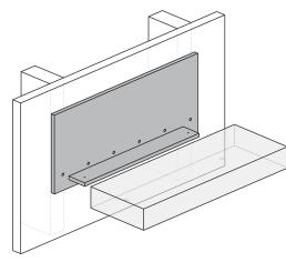
Re-install set screws with phillips screwdriver. Do not use power drill for set screw installation.
