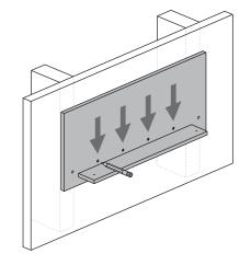
Remove bracket from wall to install wall anchors in each marked location that is not on a wall stud. Predrill each wall anchor location with 1/4" drill bit to avoid breaking wall anchors.
