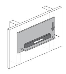
While bracket is mounted to wall, mark every remaining empty screw hole with a pencil.
