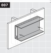
Make a final inspection of your shelf. Check for shelf sag, confirm shelf is correctly secured to wall. See **Rad Tip** ② on page 7.
