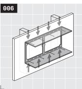
Replace the shelf and install a fastener into every location crossing a stud or blocking. For information on using the proper fastener, see Rad Tip @.
