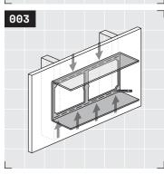
Double check the shelf position on your wall and adjust if necessary. Mark all fastener holes with a pencil. Once every fastener location has been marked, uninstall both fasteners and remove your shelf from the wall. Take a swig of your favorite soda or non-alcoholic brew.
