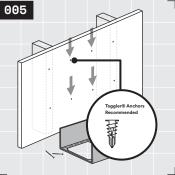
Install a drywall anchor in each of these pre-drilled locations. If you are using your own anchors, we recommend Toggler brand for best results. Stud locations should not be pre-drilled. Drywall anchors should be installed flush with the drywall surface.
