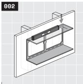
Level your shelf, then set another fastener in the next stud or opposite side with your drill. If you have installed blocking behind the full length of your shelf, skip to step 6. If you have not installed blocking, proceed to step 3. For more information on blocking, see Rad Tip ① on page 7.
