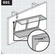
Yo! Here we go! Position your shiny new shelf on the wall in the desired location. Use a drill to fasten either the far left or right hole to the wall with the fastener holes along the top edge. For masonry installs, see Rad Tip ③ on page 7.
