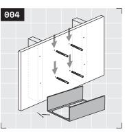
Predrill each drywall anchor location. Use a ¼" drill bit to avoid breaking drywall anchors.
