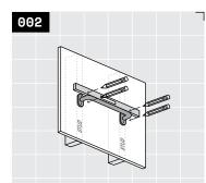
Once the structural support described in Step 1 has been established, hold the handle in desired location and mark the center of each mounting hole location with a pencil. A bubble level can be used during this step to ensure straightness.
