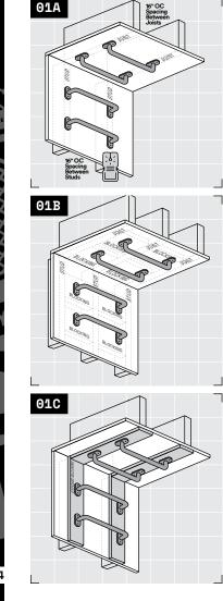
Before installation can begin, the install location must be professionally inspected and prepared with structural support as outlined in options 1A, 1B or 1C. Choose the option that best represents your structural situation and desired aesthetic. User safety is top priority. Review all warnings on page 6 before continuing!
