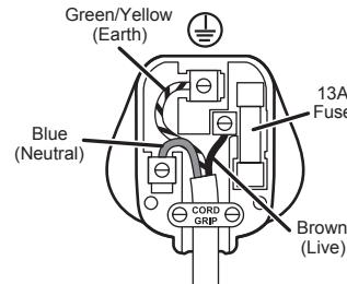
Ensure that the outer sheath of the cable is firmly held by the cord grip
