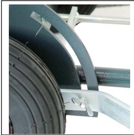
Unscrew the wing nuts and bring the right and left arm in maximum position, and tighten the wing nuts again.
