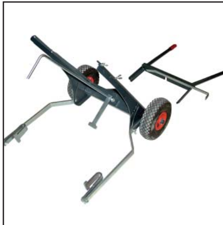
Tighten the upper part with the 4 wing nuts. Pay attention that the axle bar is correctly fitted through the cuttings.
