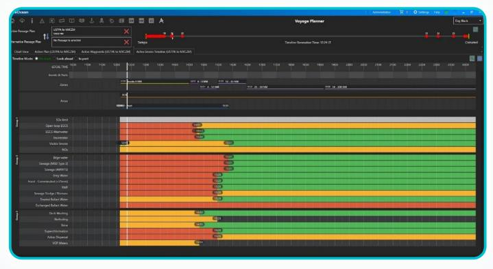
EnviroManager+'s forward-looking Environmental Timeline lists onboard operations along a a visual voyage timeline, with colour coding indicating when an action is permitted, restricted, or prohibited.
