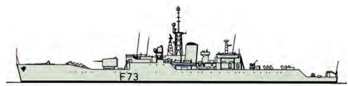
The Type 12 or Whitby class frigates were a six-ship class of anti-submarine frigates of the Royal Navy, which entered service late in the 1950s.
